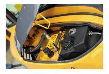
When the right hood opened, the air conditioner filter, coolant filling port, auxiliary water tank, power master switch, air conditioner dryer and battery can be maintained conveniently, which saves both time and labour.
