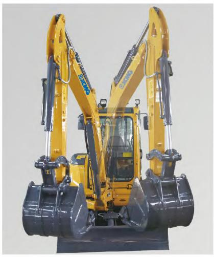
The left and right boom swing angle is respectively 75° and 50°, it can realize complex operation together with upper structure slewing to ensure that the digging is parallel with wall surface in narrow space through the cooperation of upper structure slewing so as to easily deal with various operating conditions.
