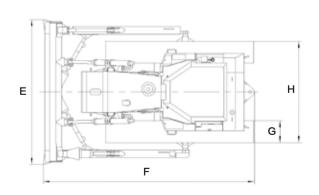
Ground clearance 离地高度.......400mm
