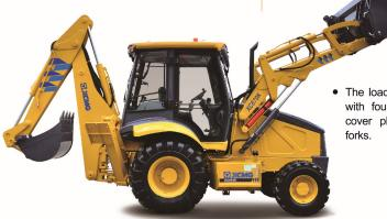
The loading end can be equipped with four-in-one bucket, manhole cover planer, snow shovel, and forks.
